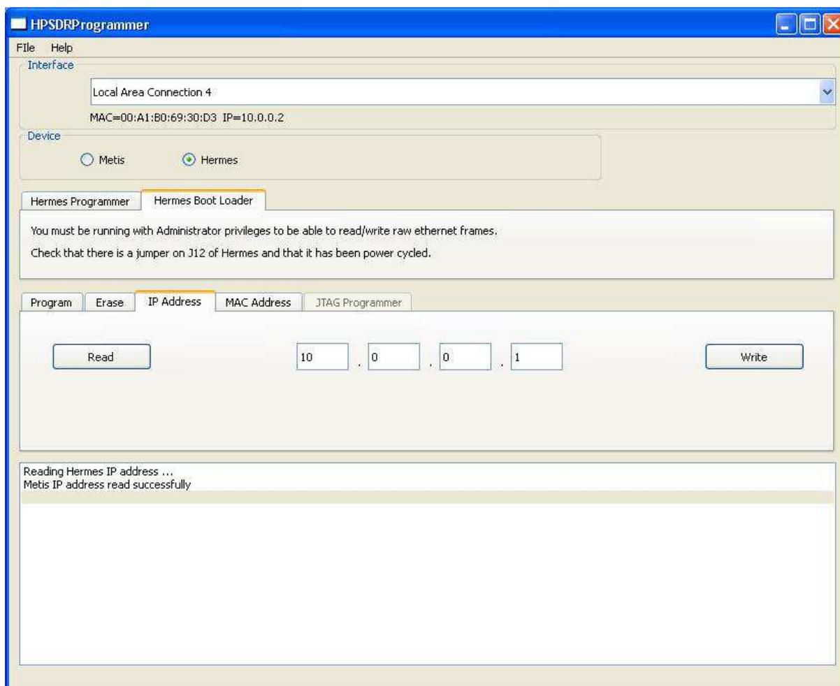
Remove the power from Hermes then remove the jumper on J12. Re-apply power to Hermes.
