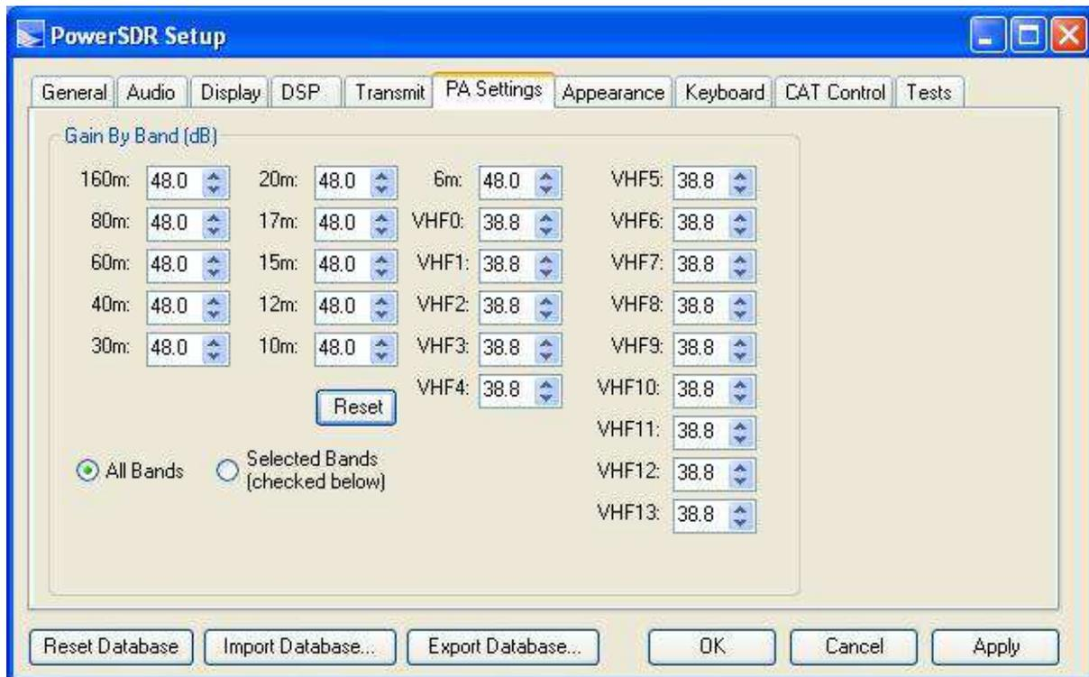
Increasing the values, indicating a higher power amplifier gain, reduces the power output.
