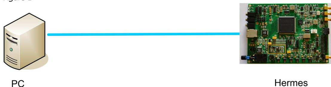
For direct connection of Hermes to a dedicated Ethernet port, a CAT 5 Ethernet cable is used. Note that a 'crossover' cable is *not* necessary but can be used if desired.
