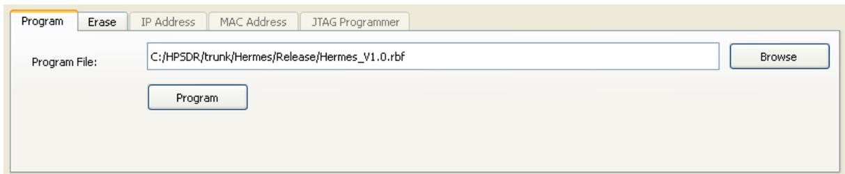
Click on the 'Program' button to start the erase and programming cycle. A successful erase and program will be indicated as follows:
