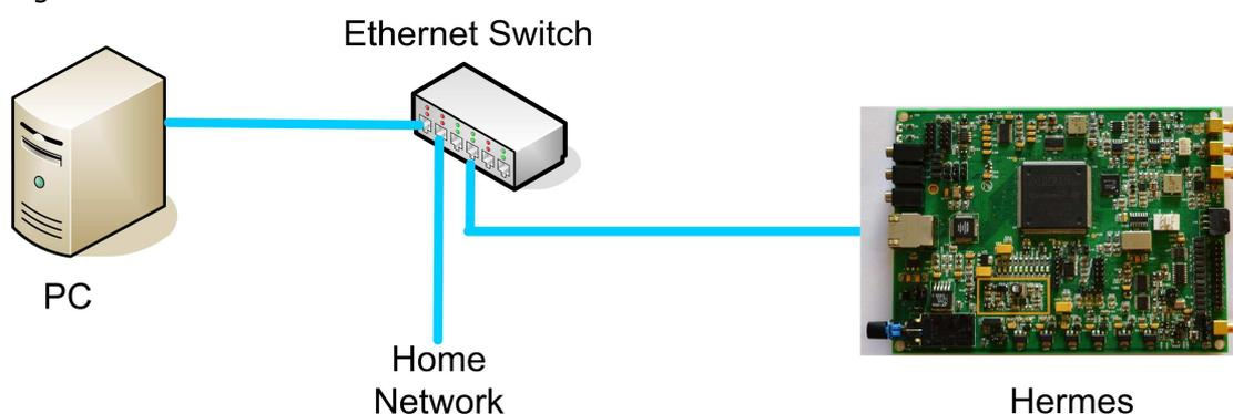
For connection of Hermes to an Ethernet switch, a CAT 5 Ethernet cable is used.
