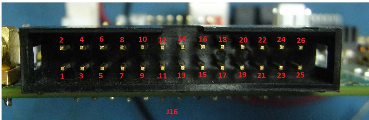
**J16:** Provides for a number of inputs and outputs as follows:
