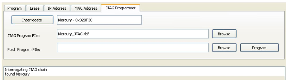
The program will automatically select the default JTAG program file; Mercury\_JTAG.rbf or Penelope\_JTAG.rbf. Should a different file be required then use the 'Browse' button to locate it.
