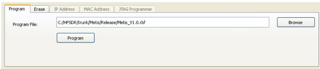
Click on the 'Program' button to start the erase and programming cycle. A successful erase and program will be indicated as follows:
