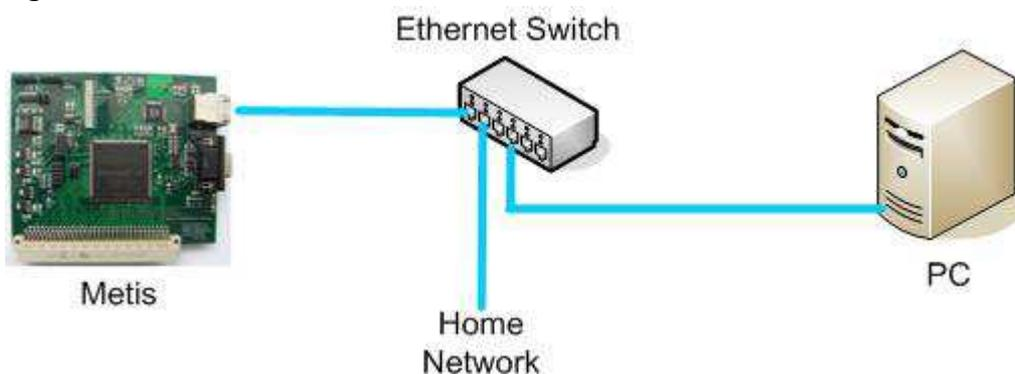
For connection to an Ethernet switch a CAT 5 Ethernet cable is used.
