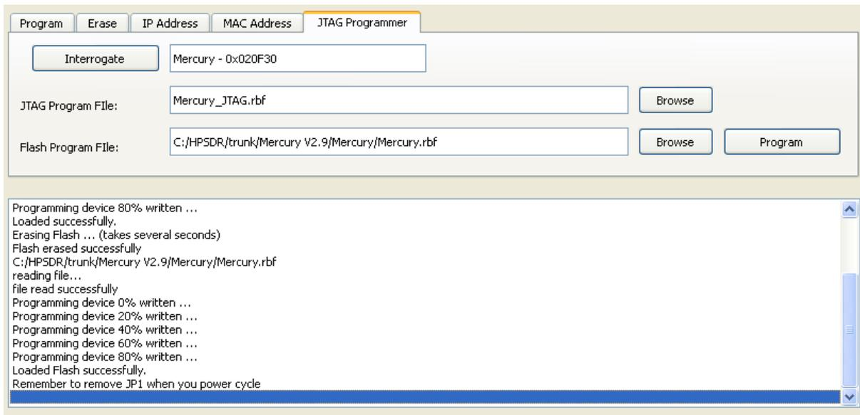
Remove power from the Atlas bus and remove the Jumper from JP1 on the Metis board. Reapply power to the Atlas bus and the new code will be loaded into the target board.
