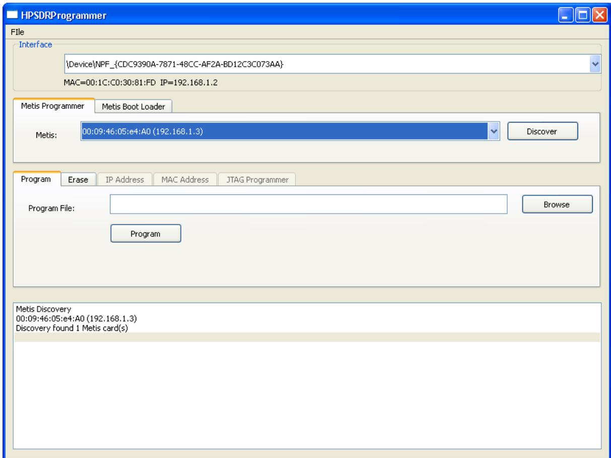
To program the selected Metis board check that the 'Program' Tab is selected. Use the 'Browse' button to locate the Metis\_Vx.x.rbf file that is to be loaded into the Metis flash memory. The current Metis\_Vx.x.rbf file can be found at <http://openhpsdr.org/download.php>.
