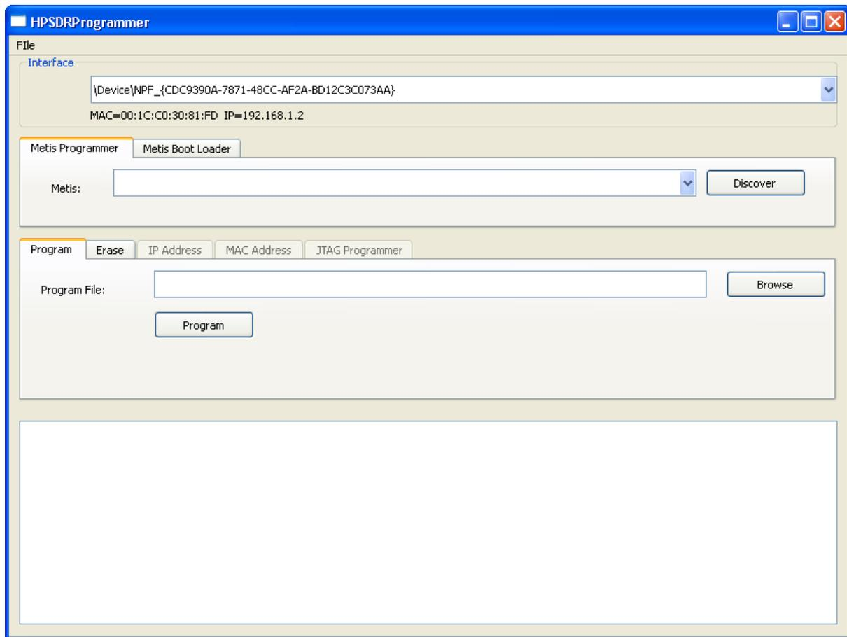
The 'Interface' section will list the Ethernet adapters present on the PC. If there is more than one found then use the drop-down menu to select the adapter that the Metis board is connected to. The IP address that the adapter is using is displayed beneath the entry to assist with selecting the correct one. The Linux version will display available adapters using eth0, eth1 etc. and MacOS X en0, en1, en2, etc.
