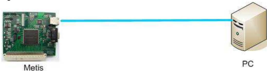
For direct connection to a dedicated Ethernet port a CAT 5 Ethernet cable is used. Note that a 'crossover' cable is not necessary but can be used if desired.
