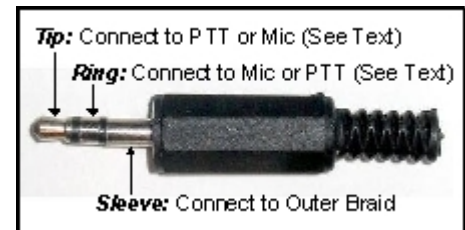
Fig 2: Microphone Plug Connections
