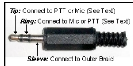
Fig 2: Microphone Plug Connections
