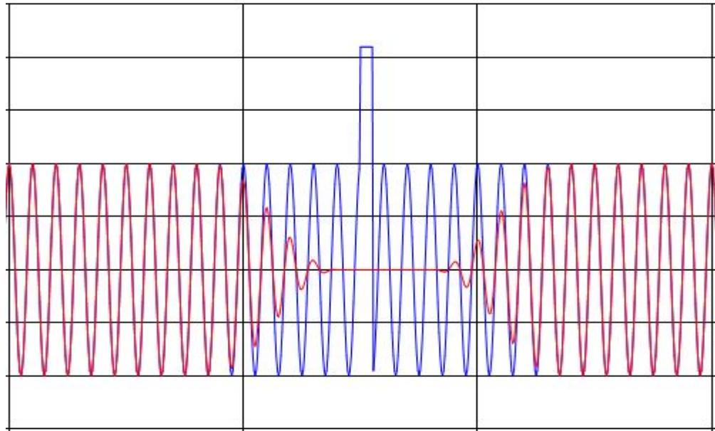
“Threshold” sets the peak level at which the input amplitude is judged to be a noise burst rather than just a signal. Therefore, if you set Threshold too low, you will begin to cut out normal signals. If you set Threshold too high, you won’t catch the noise burst.
