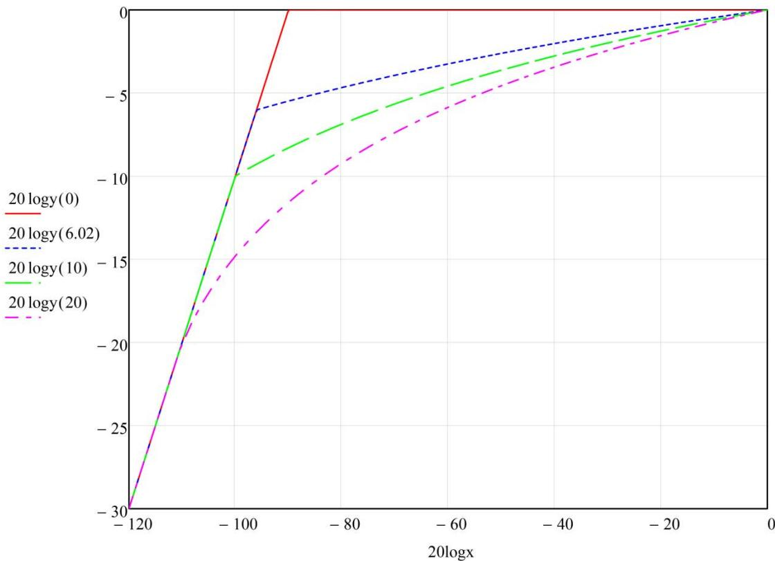
Note that if, while listening to a signal, you increase the slope setting, the volume of that signal will reduce. This is to “make room” for higher volumes of stronger signals. This effect is reflected in the above graph but may be a surprise to operators until understood.
