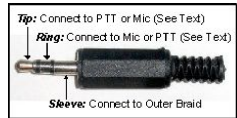
Fig 2: Microphone Plug Connections
