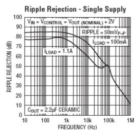
provisions. In the graph below (source LT3080 datasheet from Linear Technology) it can be seen that the ripple rejection at frequencies around 200 kHz is still in the order of 30dB. At 100 kHz it is almost 50dB.
